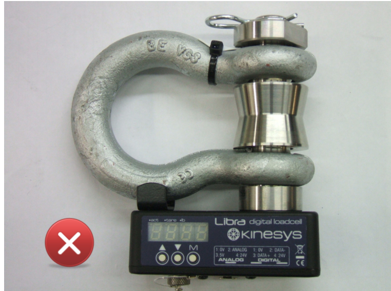
A LibraCELL with the bow fitted incorrectly.
