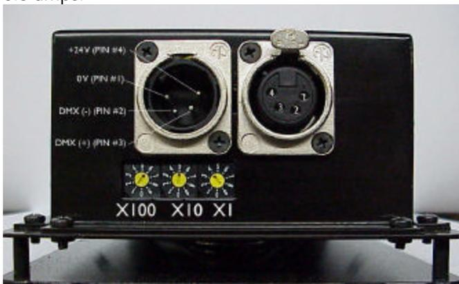
Some scroller power supplies have +24V DC on pin #1 rather than on a #4. The polarity of the pins should be carefully examined. Some manufacturers produce individual power units with two different configurations so brand identification can be misleading.
