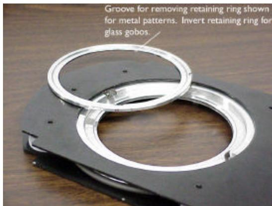
Place a small screwdriver or similar tool into the groove provided. Pry the ring upward to remove. When
