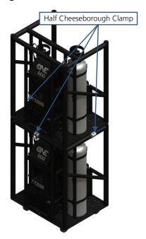
We recommend using **three** T57000 Series Half Cheeseborough from Doughty Engineering with a **Safety Work Load of 750 kg** (1650 lbs) per clamp.
